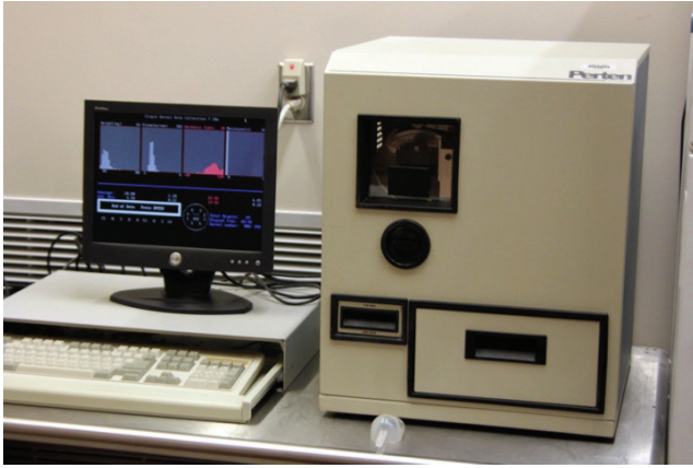
Figure 2. Pertent SKCS 4100 used to measure several physical characteristics of wheat kernels.
