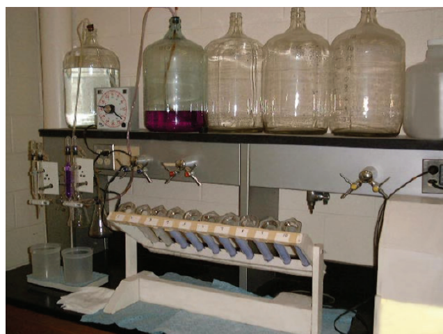
Figure 7. A sedimentation test is used to determine the quantity and quality of gluten.
